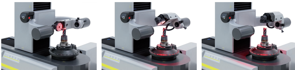
»venturion 450« with ZOLLER tool inspection. The camera can be rotated by 0° to 180° degrees.
